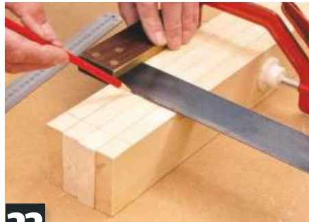
23 Doors are from 75 x 25mm PAR softwood. Saw rails to exact length but allow for waste on stiles
